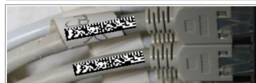
Bild 6) DMRE 8x64, 34 characters (an) for cable marking
