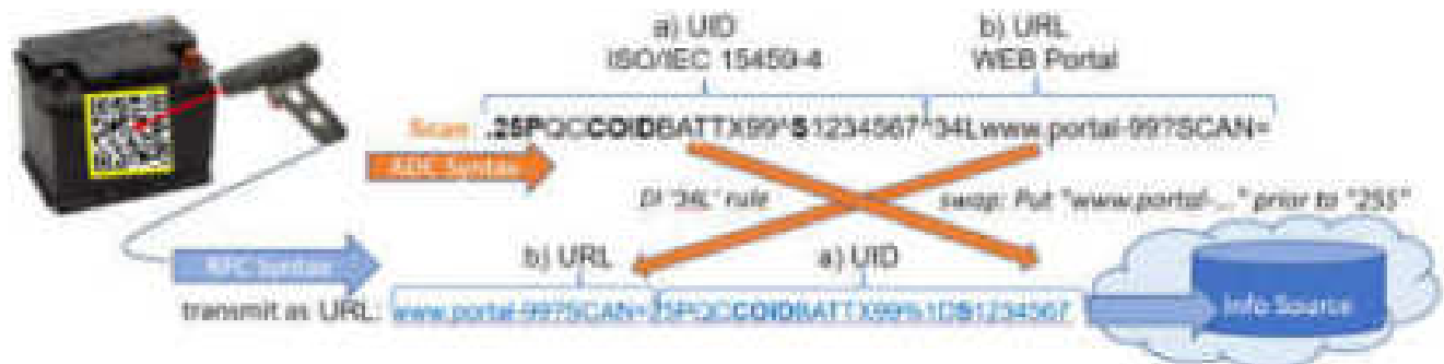
Figure 10 Example A “ID-first code” in ADC syntax, both for offline identification and for Internet access to the individual product data
