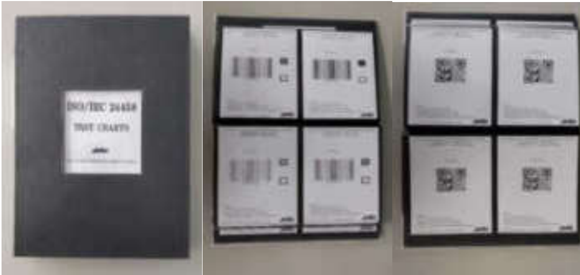
Figure 6) JAISA test chart kit includes 64 test charts for linear and 2d-bar codes
