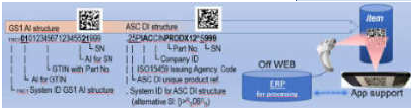
Figure 9) Two examples of “UID first” codes applied with ISO/IEC 15418 GS1 AIs and ASC MH10.8.2 DIs
