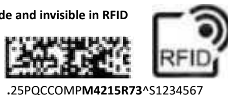
Figure 33 ISO/IEC 15459-4 conforming serialised product code in hybrid technology 2d-code and RFID
