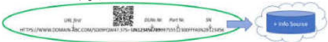
Figure 12 Example B.2.2 "URL first" according to the AutoID URL 1.3 specification with automotive-specific data elements for barcode and/or RFID and online and offline identification (Data character "+" coded as "%2B" in URL).
