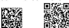
Fig. 32. Example → 5RQC... encoded with Data Matrix and/or QR Code (same dot size)
