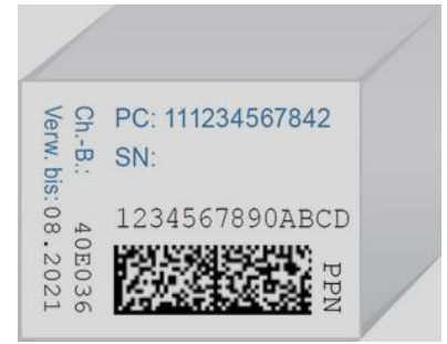
Fig. 30. Medicinal product applied with a PPN of the IFA Coding system and using DMRE.
