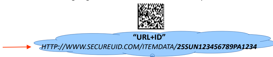
Fig. 8. Data Matrix carrying IEC 61406 Identification Link “URL first – ID after (URL+ID)”
